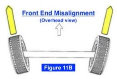
The result is easy to forecast. Your car's wheels, suspension, and front end will wear out quickly, unless they cause an accident first. Breakdown or accident, inexorably those are the only two possible outcomes of the wheel misalignment. The car will breakdown long before it ever approaches its warranty mileage.
